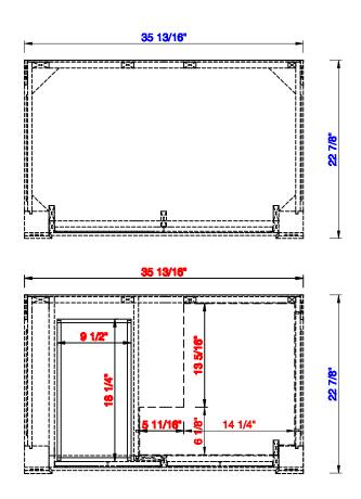
NOTE ONE: Countertops are not shown in these diagrams. (Cabinet Only) NOTE TWO: Internal Shelves (Shown) are designed to align with sinks in Ja
