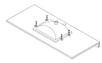
Connect a faucet to counter top. Apply a bead of silicone on the top of a cabinet (B) and place a sink (A) on it.
